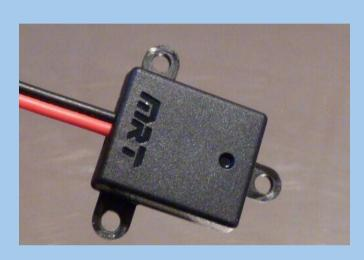
To change the mPTX number place it on a coin or other metal object, the LED should flash quickly.
